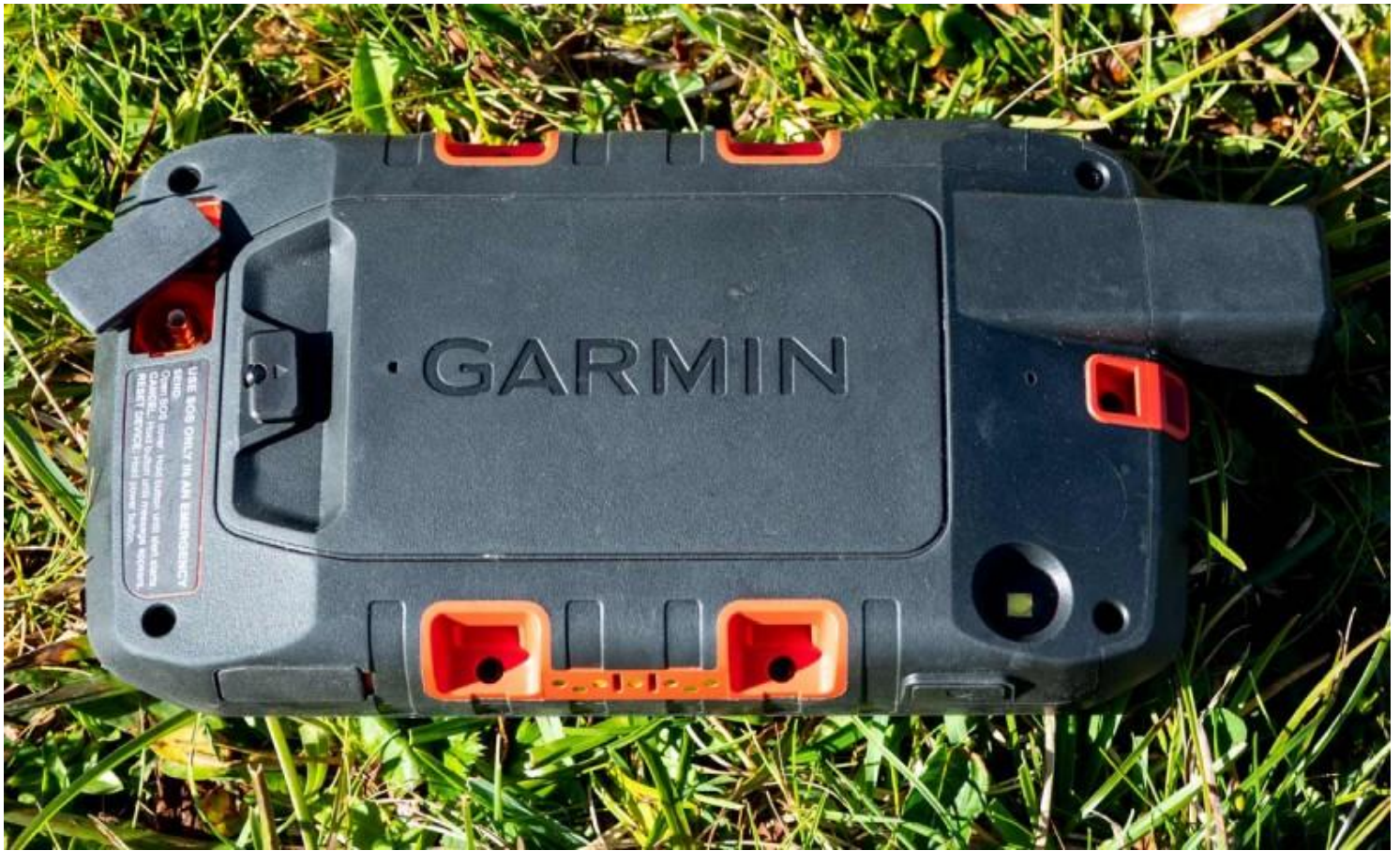
Garmin Montana 700i – rear side (top left: MCX connector; bottom left: micro USB port)
